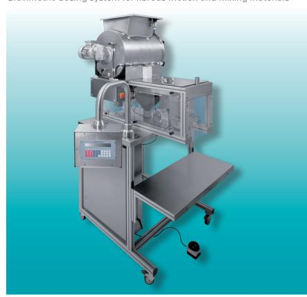
The gravimetric batch weighers of the series DW - T are dosing systems especially developed for mixing-and problem materials. Depending on the weigher type, the capacities are between 5g up to 5000g<sup>1)</sup> with 12 weighments/min and an accuracy up to 0.05%. As conveying systems belts, vibration channels, vibration belts or screw conveyors are at your disposal.
